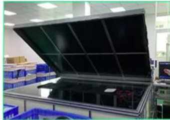
EL testing for foldable solar panel
